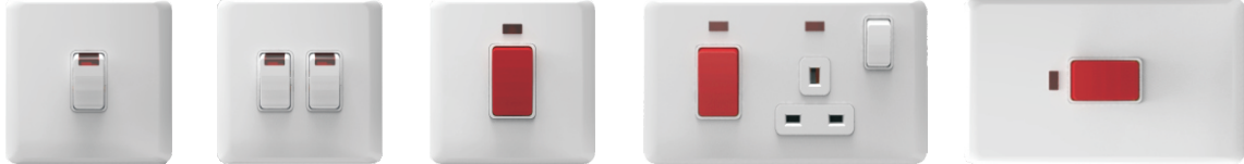
W80/20L1 1G 20A D/P Switch W/Neon W80/20L2 2G 20A D/P Switches W/Neon W80/45L1 1G 45A D/P Switch W/Neon W80/45L1/C 45A DP Cooker Connection Unit With 13A switched socket W80/45L1/B 1G 45A D/P Switch W/Neon 20AX 250V~ 20AX 250V~ 45A 250V~ 45A 250V~ 45A 250V~ 10Pcs/Box 10Pcs/Box 10Pcs/Box 6Pcs/Box 6Pcs/Box 25mm M-Box 25mm M-Box 25mm M-Box 35mm M-Box 35mm M-Box
